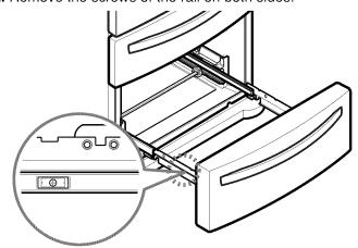
**3.** With both hands, hold both sides of the door and pull it up to separate it from the rails.
